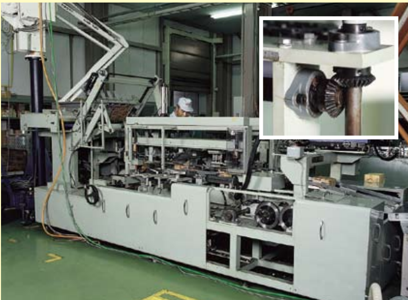
Automatic packaging machine (Spur gears) (Miter gears - inset)
